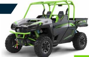
Yet there's no mistaking that a Havoc side-by-side is engineered to deliver heart-pounding thrills with 100 horsepower on tap whenever it's playtime. That power comes fast and furious thanks to the 957cc SOHC twin-cylinder, liquid-cooled EFI engine that is designed and built by Textron. It feeds its 100 horsepower and 67-ft.-lbs. of torque to a smooth and durable CVT system.
