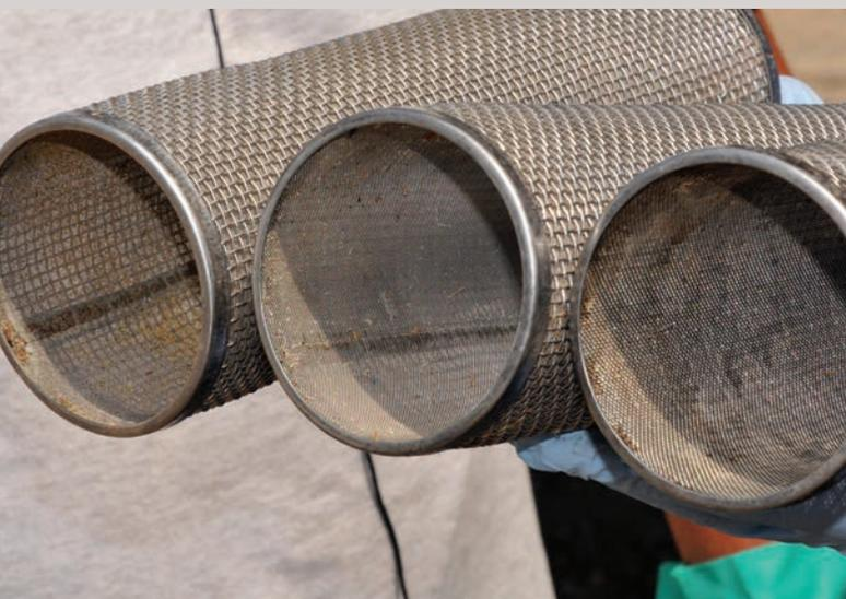
*This photo shows the differences in screen mesh size. The mesh is the fine screen under the coarse structural part of the screen.*
