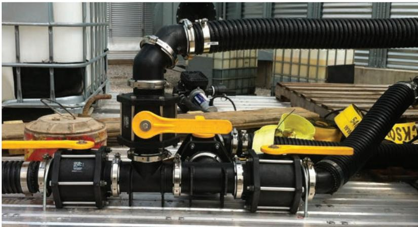
*Take care to not introduce contaminants from the trucks that fill up the sprayers. There are a lot of separate lines to flush with this setup. Open and close each valve handle as part of the rinsing process.*
