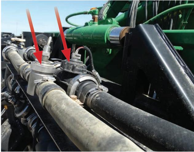
*An often-overlooked part of cleaning a sprayer is the system of hoses that move liquid through the flow meters (meters marked with red arrows).*
