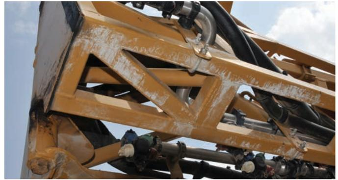
*You can readily see dried herbicide residue on the equipment (top). This operator uses a power washer to clean the outside of the sprayer (bottom).*
