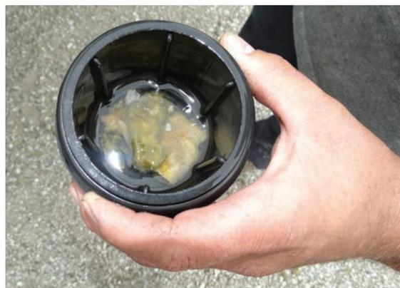
*The screen in this water tank shows a buildup of algae (above) and rust (below).*
