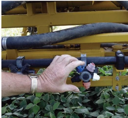
*Nozzle bodies with multiple tips need to be rotated to ensure that you flush out any trapped residue in the body. Always wear gloves during the process.*
