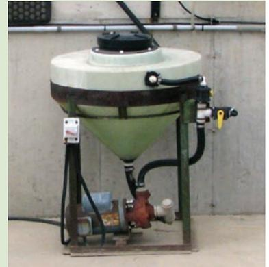
*Thoroughly clean the pumps and screens on inductor cones.*
