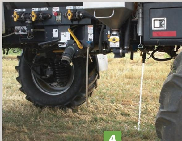
*Some application equipment may have a ball valve at the end of the screen nearest the pump (photographs 1 and 2). The ball valve allows the screen to be easily flushed when you open the valve. While opening the valve can remove a significant amount of residue from the inside of the filter, you should never just open the valve and skip manually cleaning the screen (photographs 3 and 4). The only way to thoroughly clean a screen is to remove it and to use a brush with tank cleaner and hot water.*
