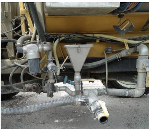
*When circulating the tank cleaner through the sprayer system, make sure to open the valves to allow the cleaning solution to move into the inductor hoses. Some applicators add a small amount of tank cleaner directly to the inductor as an extra precaution.*
