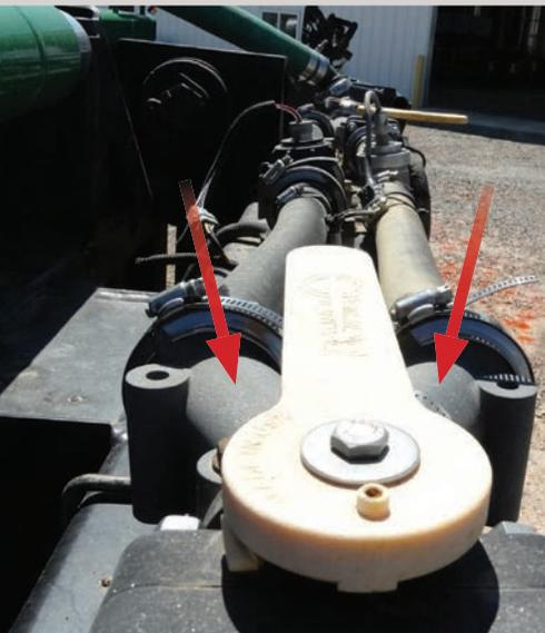
*Notice the flow then comes together at a Y junction (red arrows). Flow from one side of the Y can actually back up into the other. Unless you run clean water in each side, the remaining herbicide can become a contaminant.*
