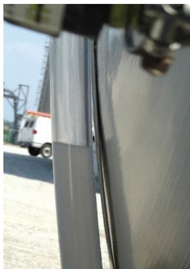
*A plastic sight gauge may help you determine if a tank has been cleaned. A cloudy sight gauge may indicate there is still herbicide residue in the tank.*
