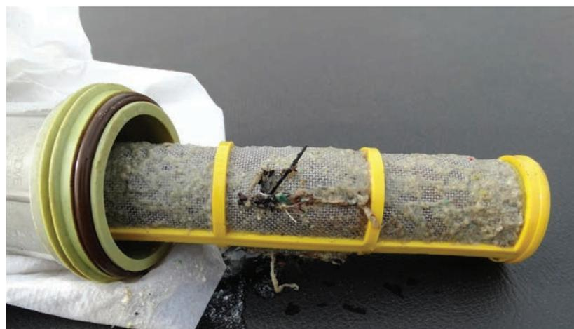
*Fewer applicators are using screens at the nozzle tips than they once did, because it takes too much time to clean that many screens. There are 96 nozzles on a 120-foot boom. Most manufacturers of new sprayers rely on the other screens to remove debris before it gets to the tips. However, for those other screens to be effective, they must be 50- or 100-mesh to do the job. Check the manufacturer's instructions — they suggest screen sizes.*
