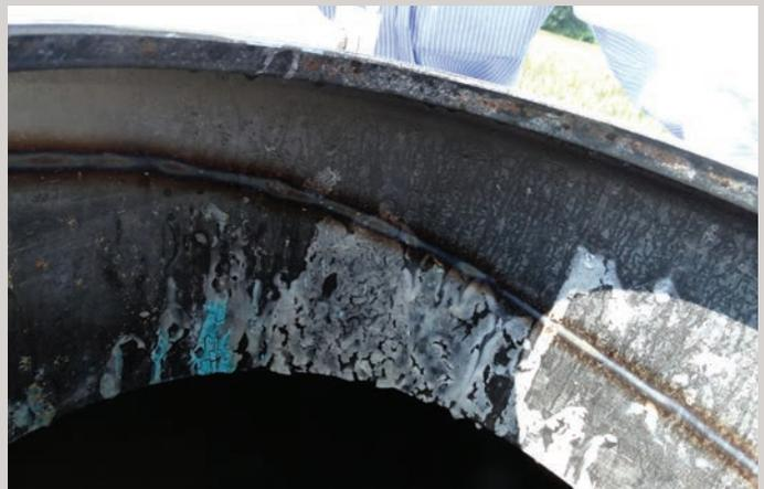
*Some tank openings have locations that the side wall cleaner and agitation device cannot fully reach (left). In this example, a piece of metal runs around the rim of the tank opening where residues have built up (right). The only way to remove this residue is with a hose or high-pressure sprayer.*
