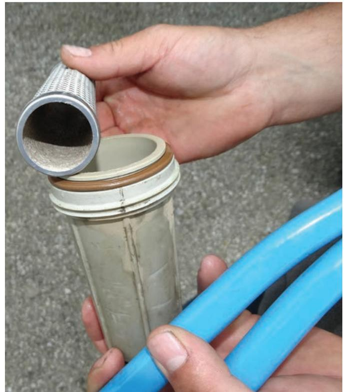
*The buildup in a screen may not always contain active herbicide. This image shows a screen with clay particles from formulations and  $\text{CaSO}_4$  from adding AMS for hard water.*
