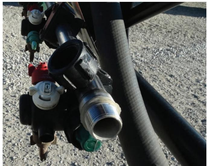
*This end cap has been modified with a quick coupler to allow for easy removal and cleanout. Make sure to use a plastic tie on the lock rings to secure the coupler.*
