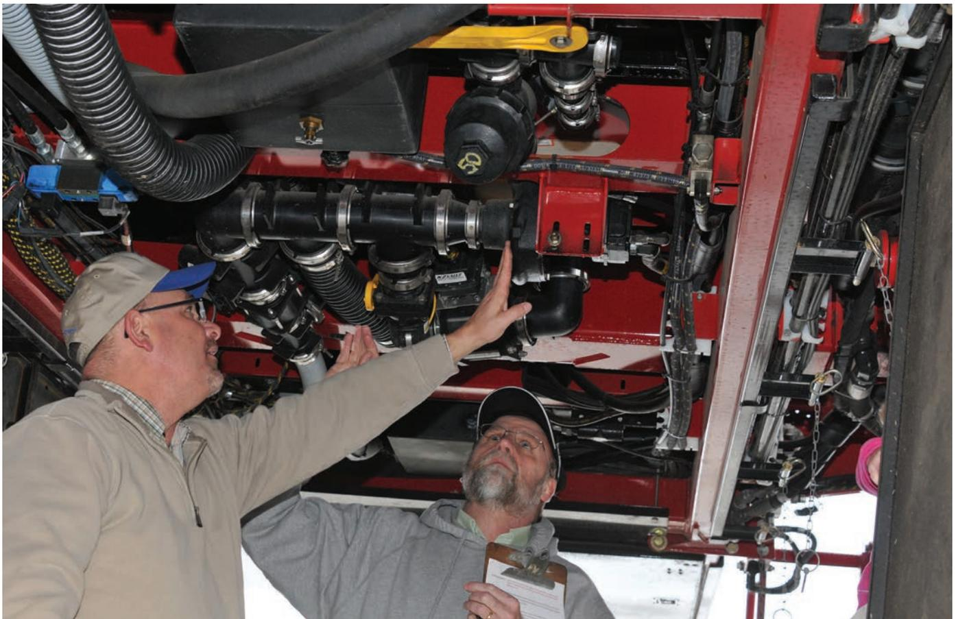
*Sprayers have complicated interconnections of hoses, filters, and valves to control flow and pressure. A standard operating procedure and cleanout checklist will ensure that you omit no step.*
