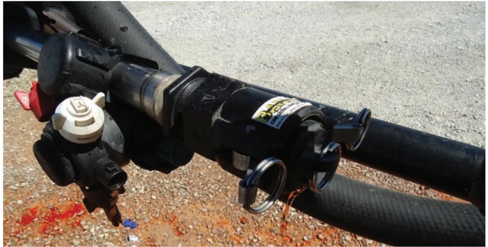
*This boom section has been modified. The owner has removed the end cap and replaced it with a valve that can flush the end of the boom.*
