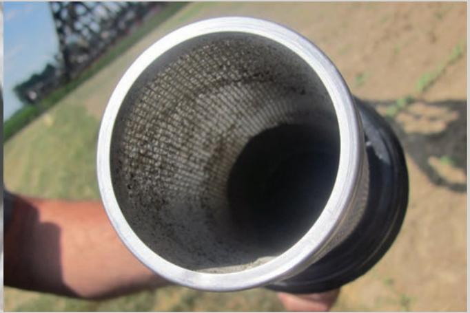
*Materials accumulated in the filter between the tank and pump (left).
