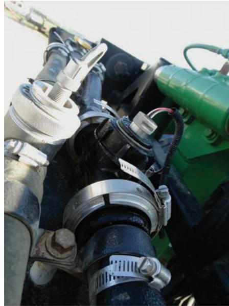
*Some sprayers are equipped with dual flow meters for high- and low-flow rates. If you do not use the second flow meter, the herbicide may get trapped on the outlet side of the valve. If you do not flush the inlet after use, it is possible that the herbicide will sit in that section until you open the valve.*
