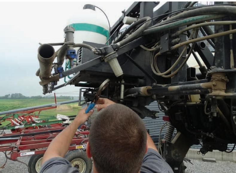
*Always wear gloves and eye protection when you work around pressurized water or air while handling screens. The screens may contain concentrated product that has not dissolved.*
