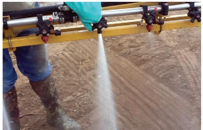
*This photo shows a 10-inch spacing sprayer between nozzles, but the producer used a 20-inch spacing. Field damage was traced back to unused nozzle clusters that had not been rinsed. They were only using a 20-inch spacing on their 10-inch nozzle arrangement boom. After they started turning the unused bodies and cleaning them out, they reduced contamination.*
