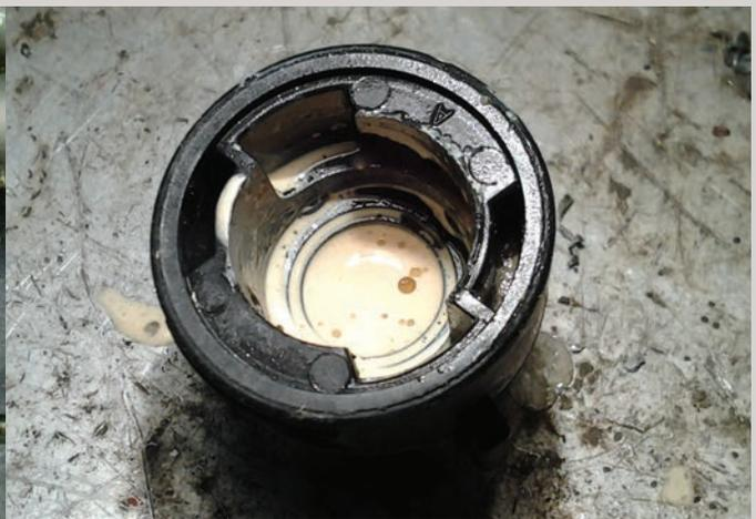
*The right photo shows herbicide residue that was left in a drop nozzle from a previous use.
