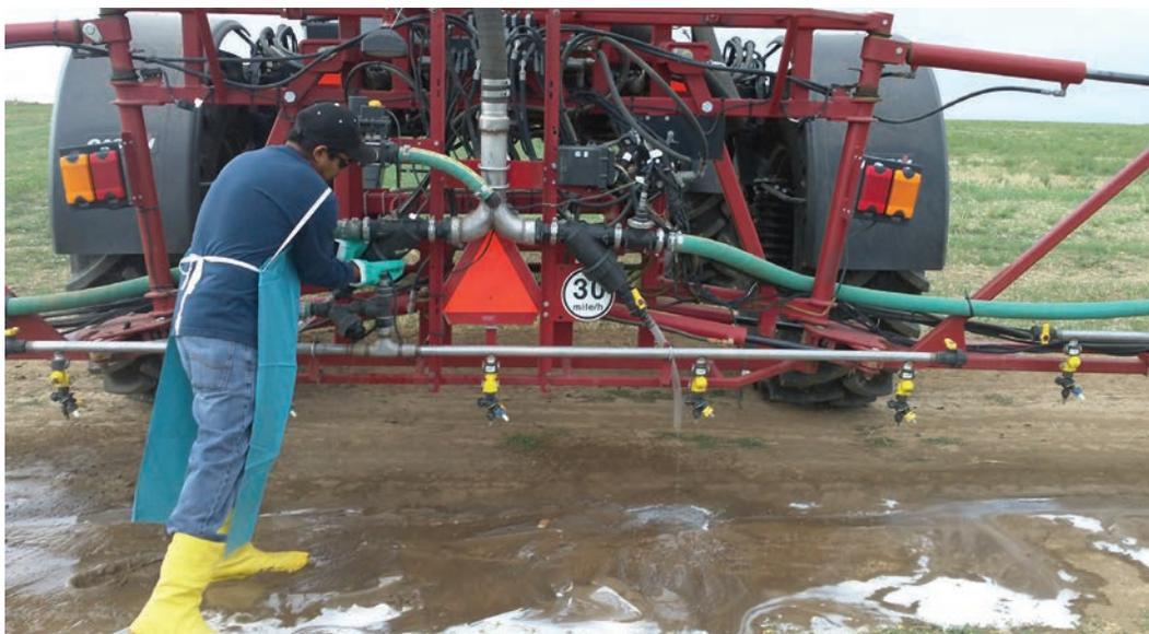
*This sprayer has two screens at the rear for each side of the boom. Note that the applicator is wearing personal protective equipment.*
