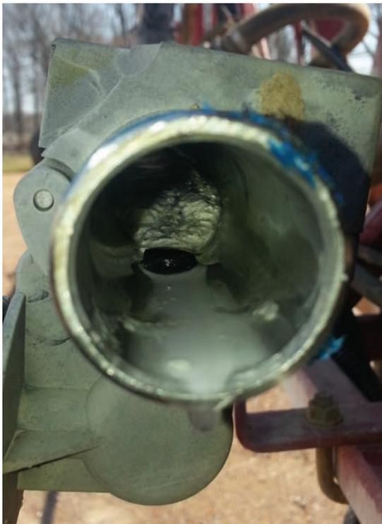
*Inside of boom after the first flush with clean water.*
