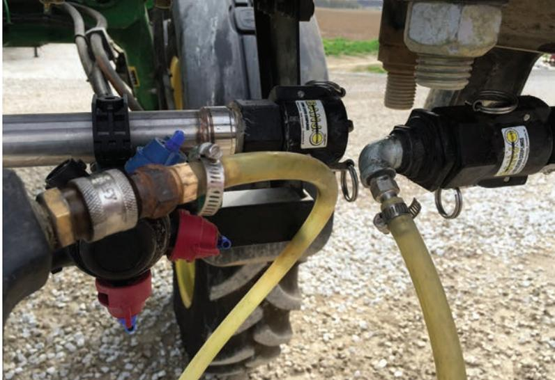
Newer self-propelled sprayer models may be engineered with an air purge system to blow out the boom sections. Normally, each boom section is purged independently. Depending on the unit, you can retrofit some older sprayer models with this air purge equipment.
