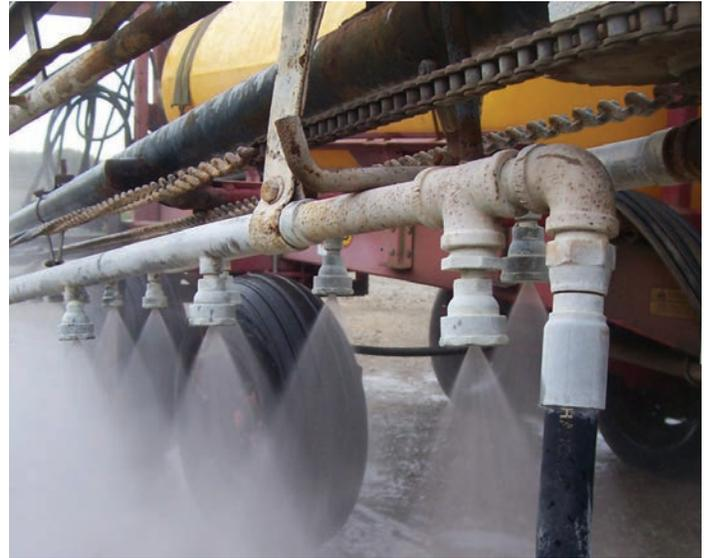
*How much water you use during the first rinse is based on experience. In all cases, water coming out of the nozzles needs to pass the eye test. In other words, water should be clear without any evidence of a tint or sheen (top). Be sure to open the end nozzle during the first flush. Continue to add water to the tank until the water exiting the nozzles is clear.*
