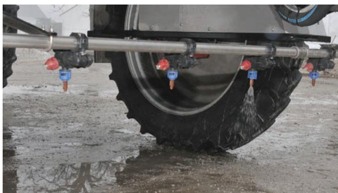
*You might think after a pump loses its prime that hardly any product would remain in the system. A 120-foot boom may hold 35 gallons of liquid, a 90-foot boom 25 gallons, and an 80-foot boom 18 gallons. Depending on the application rate, that's one to three acres of product left in the boom and hoses — a lot of potential damage waiting to happen!*
