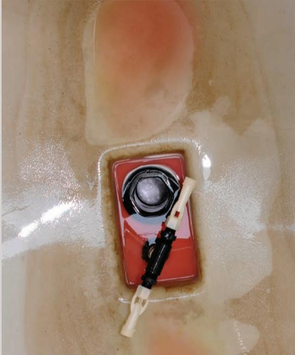
*Some tank designs do not allow complete drainage. (Left) In this case, there is liquid contained below the drain opening that the pump will not be able to pull through the system. Other tank designs allow for liquids to completely drain out of the sump (right). The first 30 to 50 gallons of clean water will remove much of the tank mixture left in the sump area and in the hoses and booms.*
