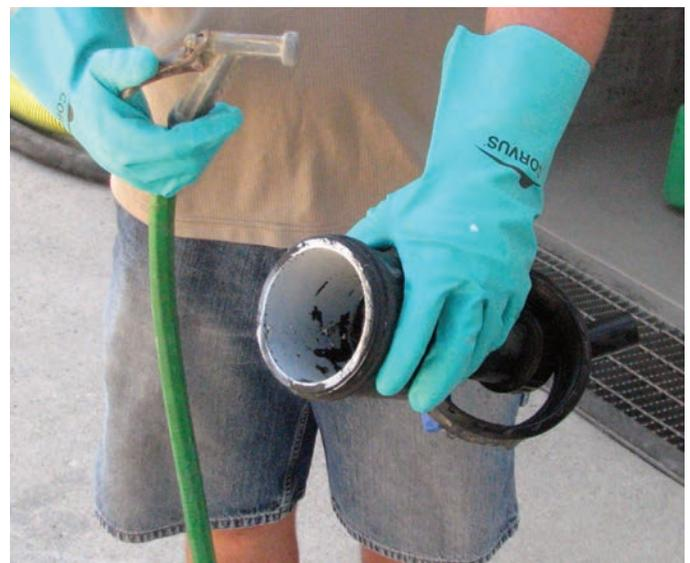
*Be sure to clean the housing that holds the filter in place, because herbicide residues can also build up on the inside walls. Use a nozzle attachment on a hose (like the one shown here) to finish rinsing.*
