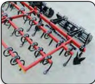
*The bedded-crop model of the Perfecta is the ideal implement for finishing beds before planting. While uprooting growing weeds to wilt and die, the Perfecta is also loosening and aerating the soil for optimum seed-to-soil or root-to-soil contact. Models are available for a variety of bed widths.*
