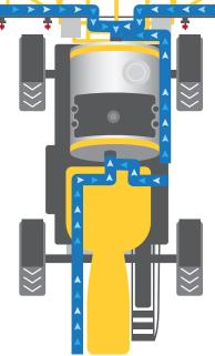
Rain, wind and a hundred other things can stop a job before it's done, letting residues settle in the plumbing. ClearFlow<sup>TM</sup>, the industry's first full-recovery system, pushes unused product from the plumbing back into the tank, prior to a tank or boom rinse. Product goes back in the tank to be reagitated or off-loaded, minimizing waste and contamination. So you'll be confident plumbing and booms are clean.
