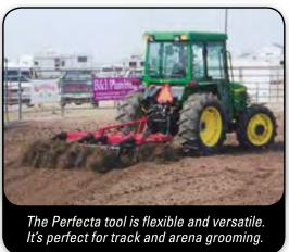
The Perfecta field cultivator is lighter, pulls easier, covers more acres and is more versatile than a comparable-sized disk. The horsepower requirement is 4-7 hp per foot. It's available in a variety of configurations, working widths from 4' to 28' and your choice of a durable, high-gloss red or green powder-coat finish.
