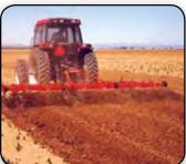
The bedded-crop model of the Perfecta is the ideal implement for finishing beds before planting. While uprooting growing weeds to wilt and die, the Perfecta is also loosening and aerating the soil for optimum seed-tosoil or root-to-soil contact. Models are available for a variety of bed widths.
