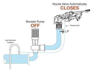
Booster Pump **OFF** (equal pressure): Delta P pressurizes the line leading to the actuator on the nozzle valve, maintaining the **VALVE CLOSED**.
