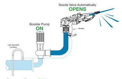
Booster Pump **ON** (pressure differential *greater than 15psi*): Delta P vents the actuator on the nozzle valve, **VALVE OPEN**.
